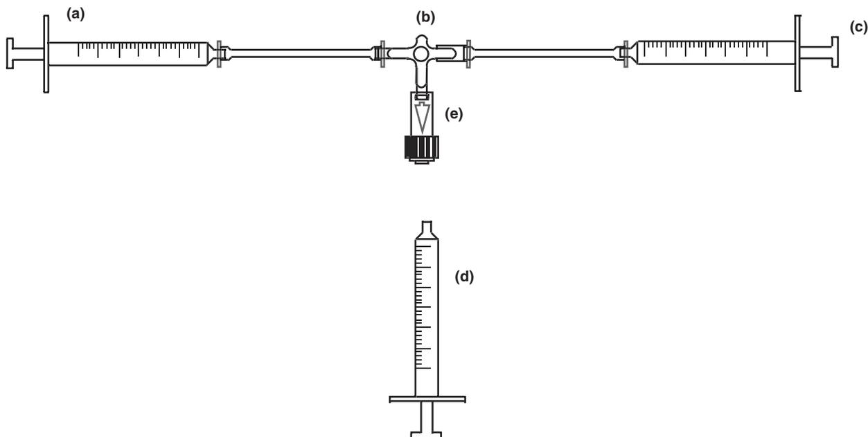
**Figure 2** Schematic diagram of the system used to assess bacterial contamination during sampling with a three-way tap or the Needle-Free Arterial Non-Injectable Connector (NIC). a – flush syringe; b – three-way tap; c – ‘patient’ syringe; d – syringe (discard/sample/waste) connected either directly to side port of three-way tap, or to e – NIC. See text for details.
